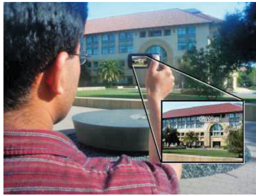
Figure 1. A snapshot of an outdoor mobile visual-search system. The system augments the viewfinder with information about the objects it recognizes in the image taken with a phone camera.
